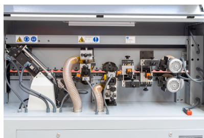
Kleben gluing Kantenanschnitt head and end cutting Doppelfeinschliff fine trim Zuführungsaggregat feeder Polieraggregat polishing unit Absaugaggregat dust collector unit
