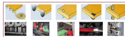
Kleben gleitend Kantenendschnitt end cutting Doppelflächenaggregate finishing K side Ziehklängenaggregate flat scraper Rollenaggregate buffing
